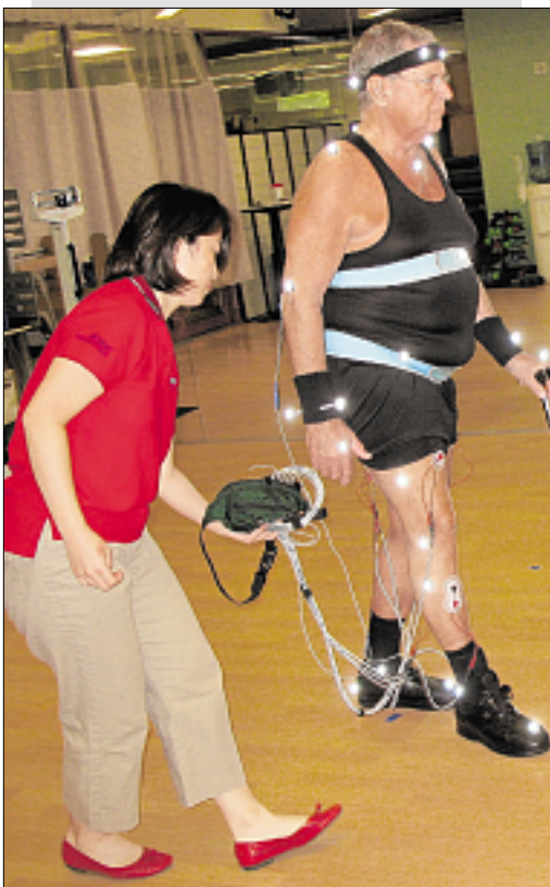
Phil Whitacre has his gait analyzed under the direction of IML biomedical engineer Dr. Akiko Mori (above); at top is how the gait analysis looks when it is computer animated.
